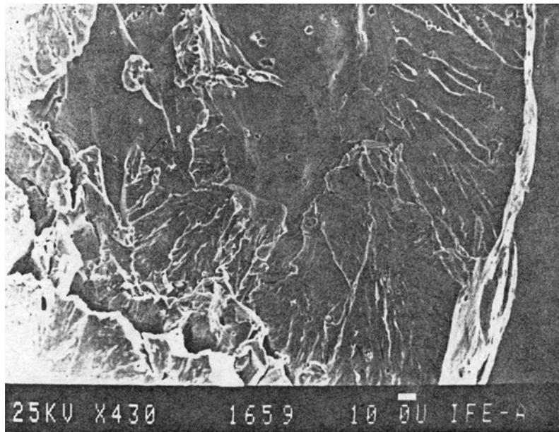
Fig. 6. Intergranular and transgranular fracture surface of aged and precharged FeO-Al<sub>2</sub>O<sub>3</sub> specimen
