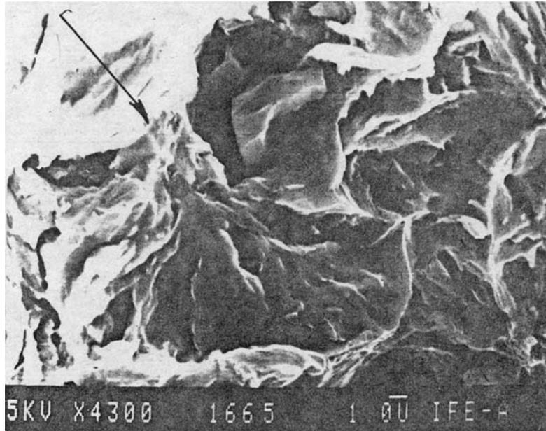
Fig. 5. Fish eyes seen on surface of aged and precharged FeO specimen
