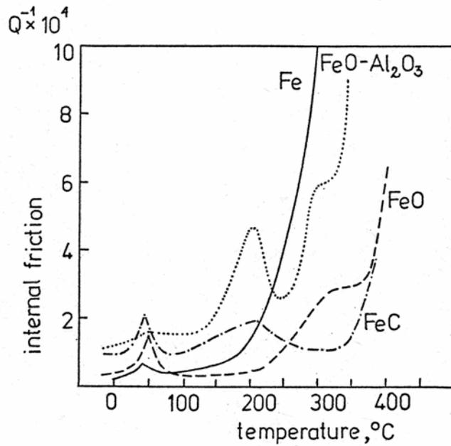
Fig. 1. Internal friction spectrum for studied alloys aged at 600 °C
