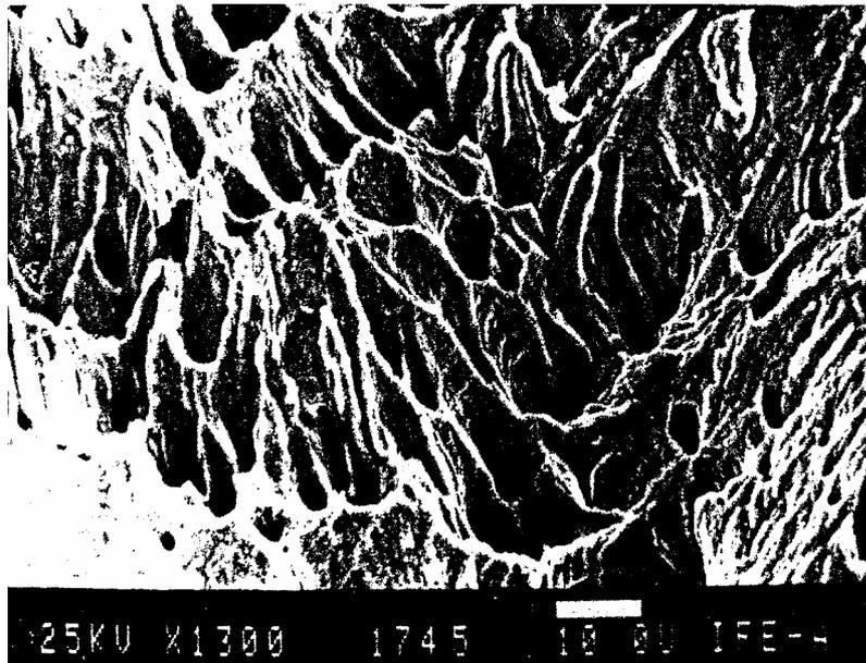
Fig. 4. Modified ductile fracture of cold worked FeO-Al<sub>2</sub>O<sub>3</sub> specimen hydrogen charged during tensile test
