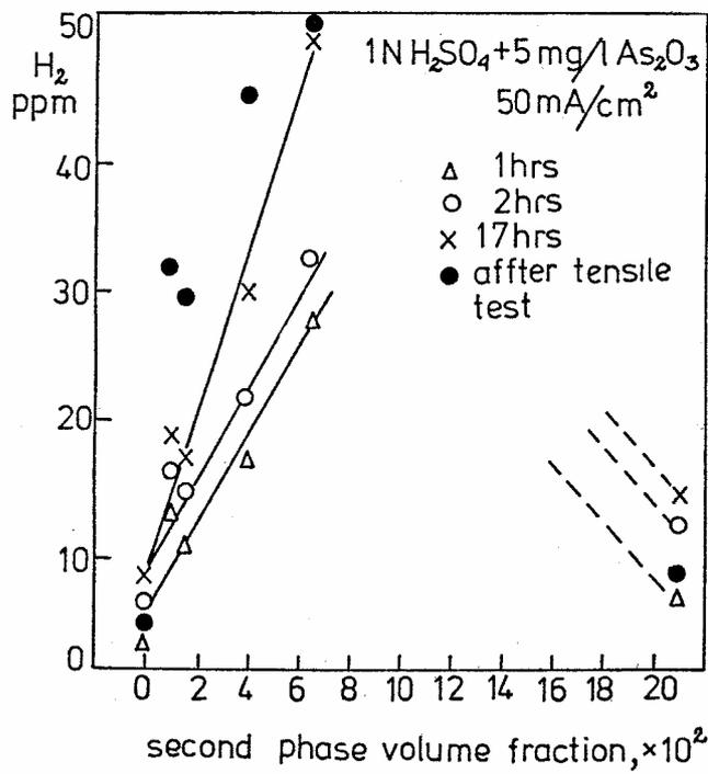
Fig. 2. Amount of hydrogen absorbed by unstressed specimens charged for different time and by specimens charged during tensile tests vs volume fraction of particles
