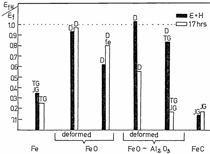
D- ductile fracture ; fe.-fish eyes
